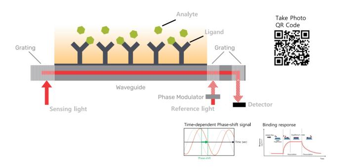
Grating-Coupled Interferometry (GCI) is a surface-based, label-free biosensing technique.
