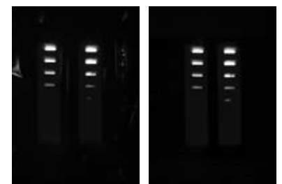
Figure 2. Use of a background quenching sheet under a chemiluminescent blot reduces noise that results when stray light scatters off plastic wrap.
